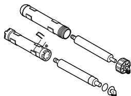
6. Remove cap (unscrew tubing first—on some models). Use pliers to remove the RO Cartridge. Place in a clean plastic bag or discard if replacing. Thoroughly wipe inside of housing and cap with a paper towel or dish brush moistened with dish soap. Rinse well.
