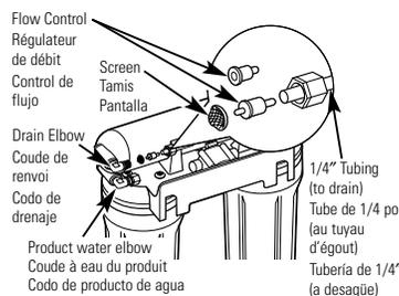
13. If you replaced RO cartridge, also replace flow control and screen. (Remove flow control with clean knife edge. Remove screen with a clean toothpick.)
